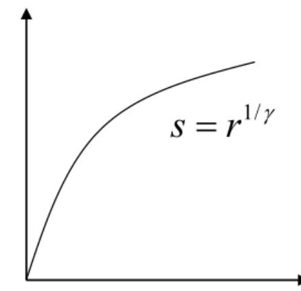
$$\begin{aligned}i &= s^\gamma \\&= (r^{1/\gamma})^\gamma \\&= r\end{aligned}$$
