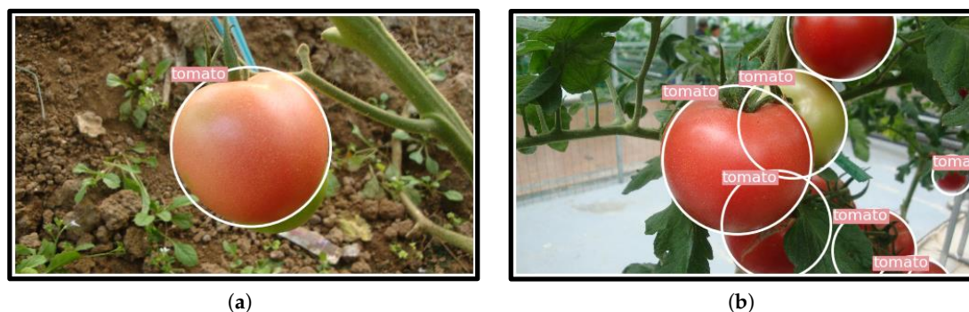
Figure 15. Some missed detection results due to severe occlusion by leaves or other tomatoes: (a) the green tomato which was largely covered by the red one was not detected, and (b) the red tomato was missed due to severe occlusion by leaves, stems and other tomatoes.
